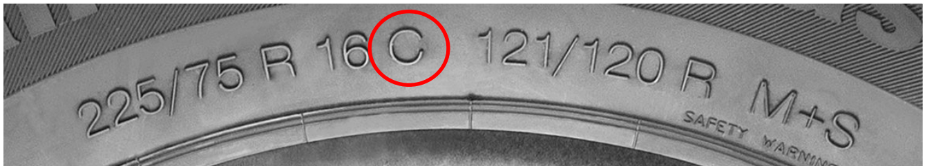
FIGURE 3: Size and Service Description of an Example C-Type European Commercial Metric Tire
